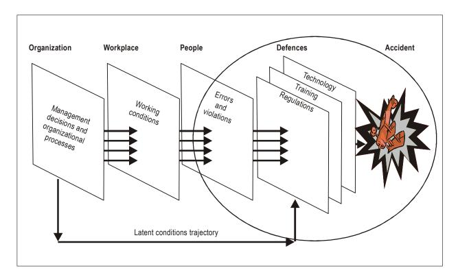
Figure 2-2. The concept of accident causation
