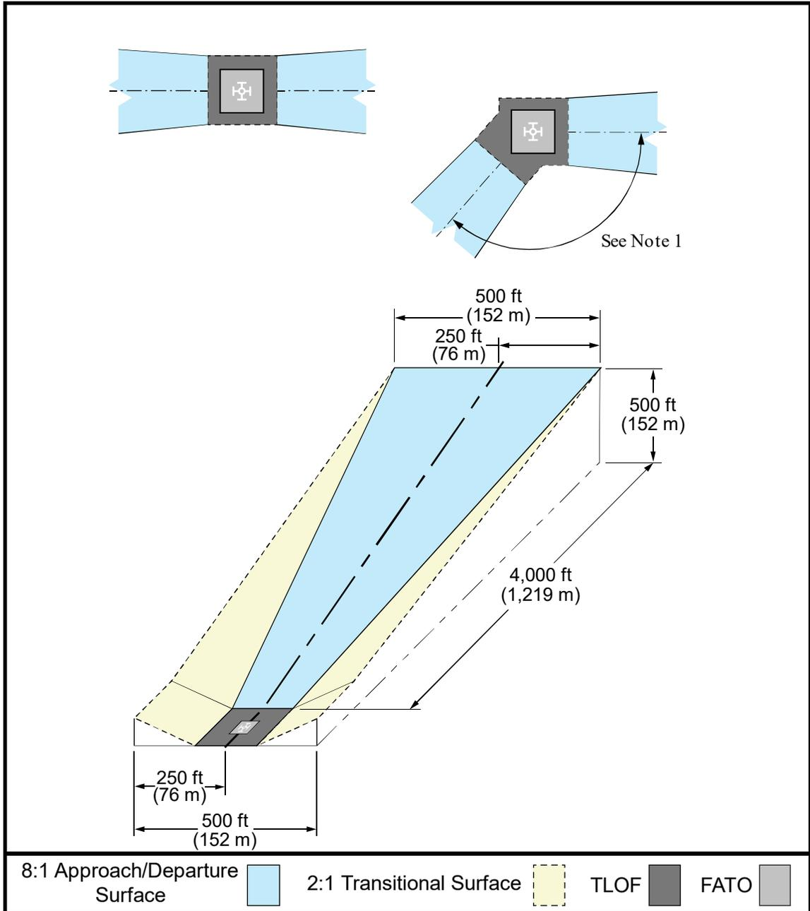
**Note 1:** The preferred approach/departure surface is based on the predominant wind direction. Where a reciprocal approach/departure surface is not possible in the opposite direction, use a minimum 135-degree angle between the two surfaces.
