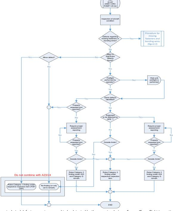
NOTE: Some technical defects are not supposed to be detected by the operator during a "normal" pre-flight inspection and should therefore not constitute a finding. Examples of such defects could be:
