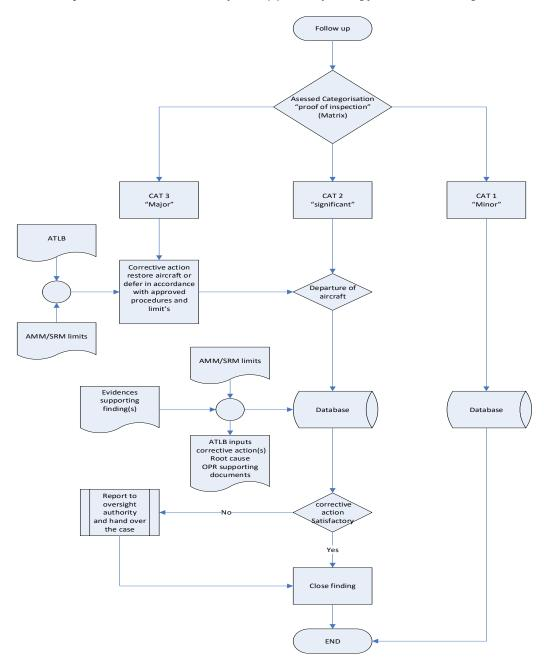
Note: Standard Class 1 action process applies for category 1 findings related to fasteners and bonding wires.
